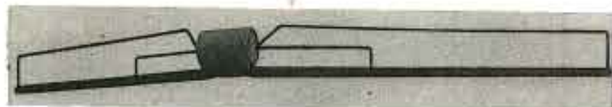
Figure 3 Cathode-follower dipole for the television bands.
